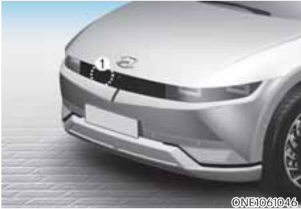
[1]: Front radar For detail location of sensor, refer to the picture above.
